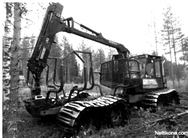
Fig.4: Typical 8-wheeledforwarder on Finnish peatlands.
